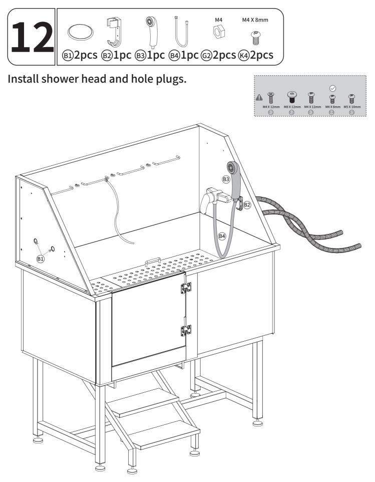
Please apply waterproof tape to the connections of the water pipe for waterproofing protection.
