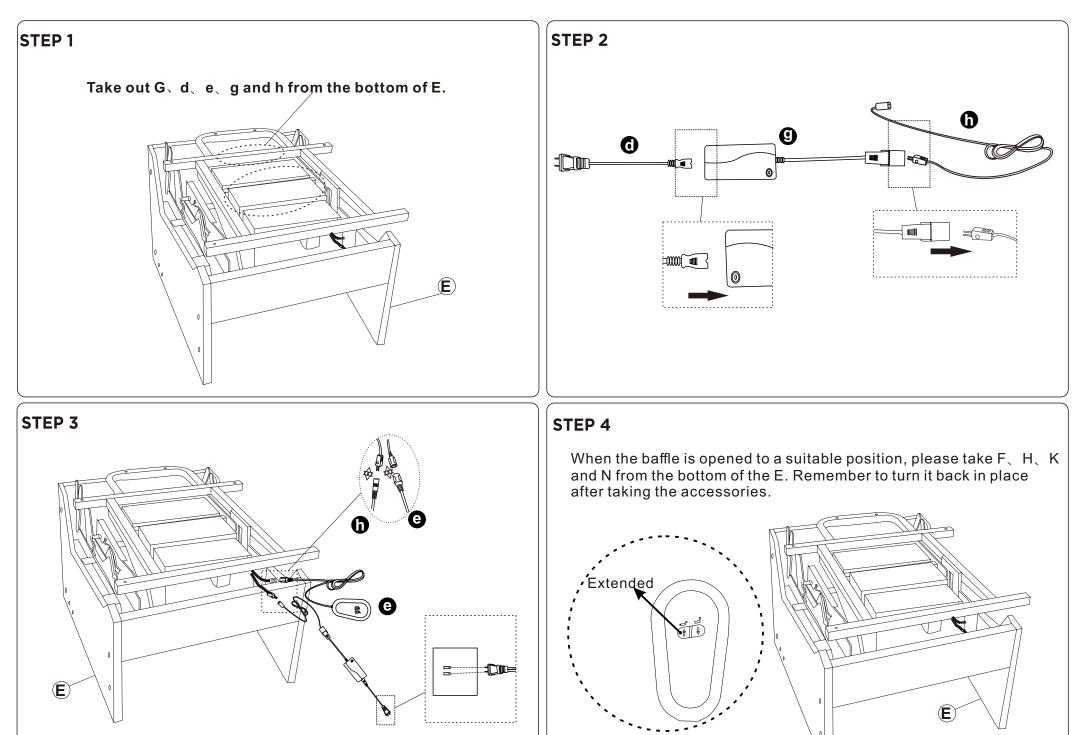
The Extension Cord and the Remote Control connect the corresponding power supply and remote control interface of the bottom of E , and the insert the socket.
