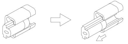
You can pull the buckle out by following the direction indicated by the arrow
