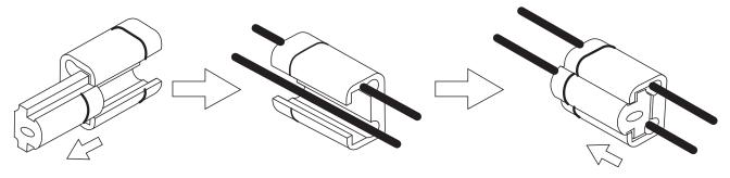
You can pull the buckle out by following the direction indicated by the arrow
