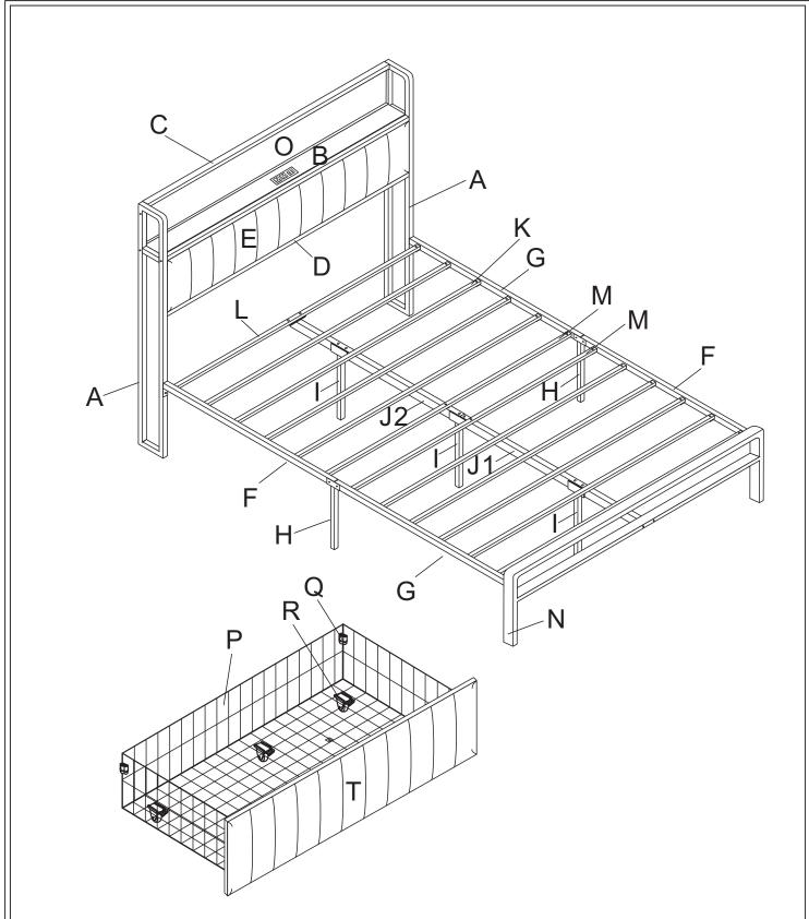
Notice: Do not tighten the screws too tightly at the beginning of the assembly. After each hole position is matched well, apply gentle force to screw, if there is no problem, then tighten all the screws.
