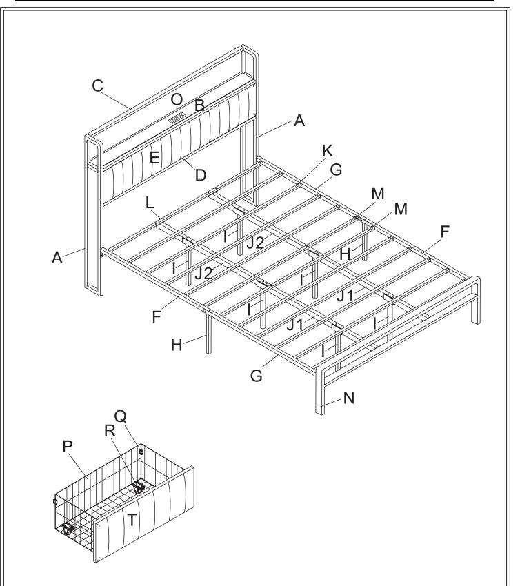
Notice: Do not tighten the screws too tightly at the beginning of the assembly. After each hole position is matched well, apply gentle force to screw, if there is no problem, then tighten all the screws.
