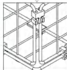
The plastic buckle is placed between the two wires as shown.
