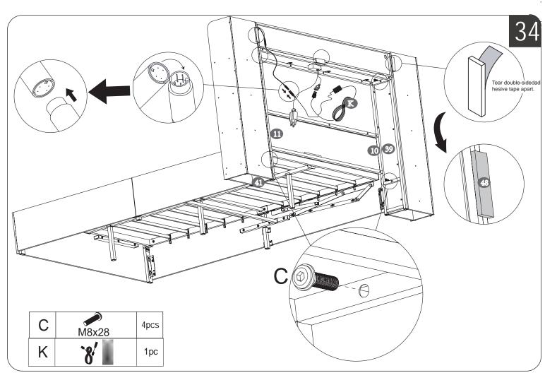
If you do not wish to use the storage cabinets on either side of the headboard, you can remove them by unscrewing the screws.
