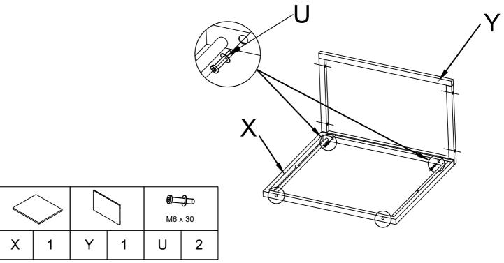
Please DO NOT tighten the screws at this step yet. Wait to tighten all the screws until the product is fully installed.
