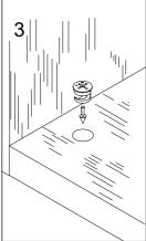
Turn the female camlock clockwise with a screwdriver.
