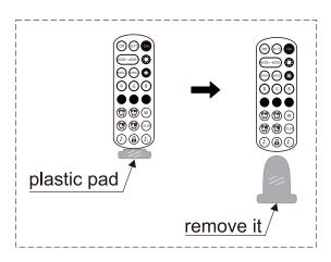
Remove the plastic pad on the remote control after the installation was complete and start the remote operation without direction restriction.
