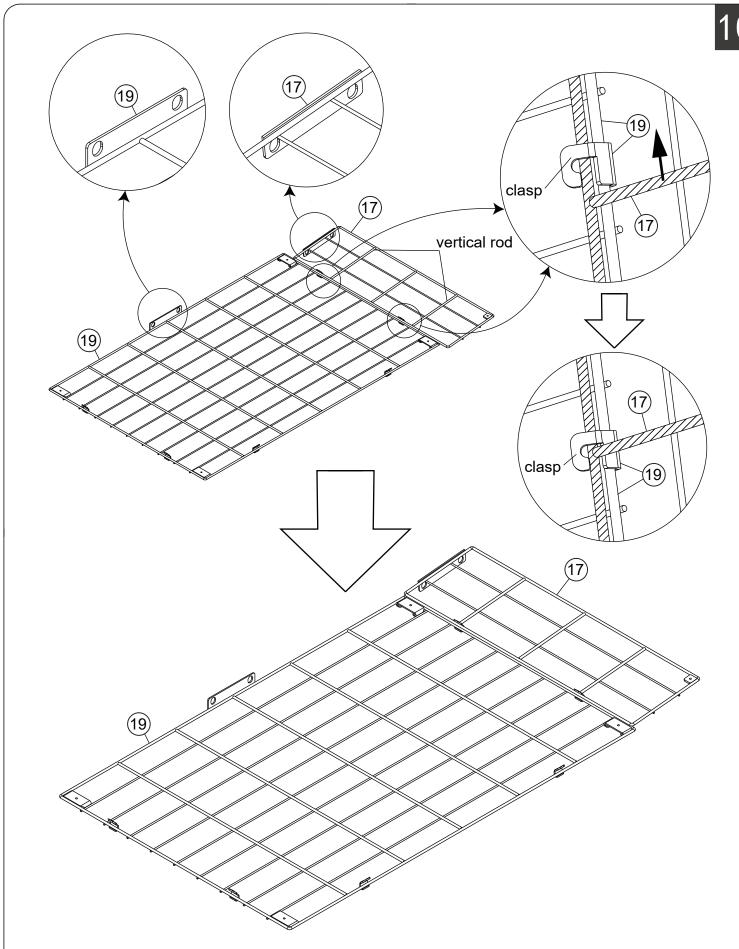
NOTE:Push component 17 lying flat into the clasp of component 19 until the vertical rod of component 17 is against the clasp
