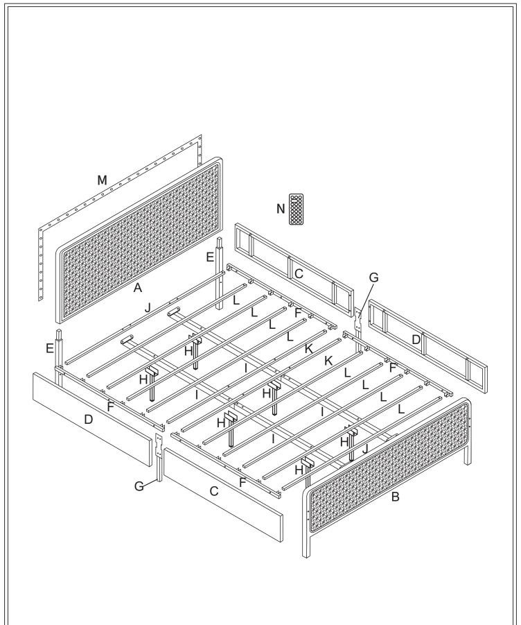
Notice: Do not tighten the screws too tightly at the beginning of the assembly. Wait until all the hole positions and screws are matched, then gently tighten all the screws.
