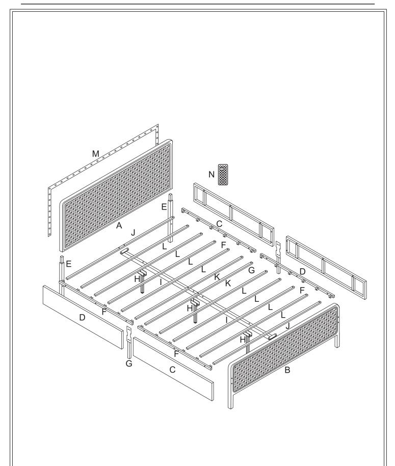
Notice: Do not tighten the screws too tightly at the beginning of the assembly. Wait until all the hole positions and screws are matched, then gently tighten all the screws.
