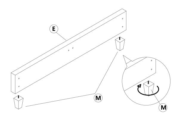
4 Loosen the screw of siderails, install the edge of the foot, and tight the innerscrew.
