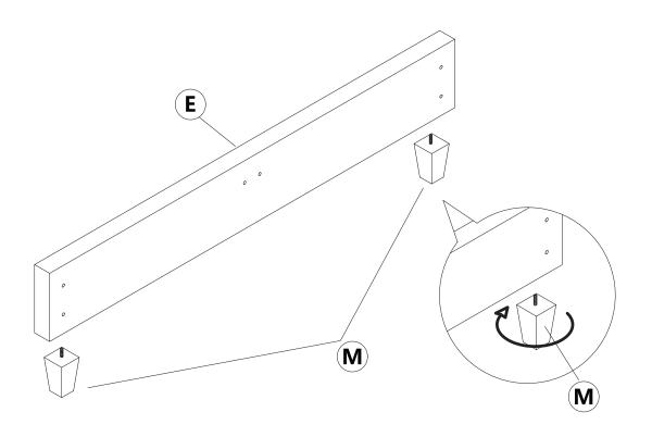
Loosen the screw of siderails, install the edge of the foot, and tight the innerscrew.
